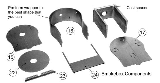
9. Secure the smoke box front (part 15) to a block of wood using drawing pins and solder the wrapper (part 16) around the edges so that the front acts as a former. Start by positioning the wrapper to the centre of the smoke box front top, there being a small half etched centre line mark to aid positioning.
