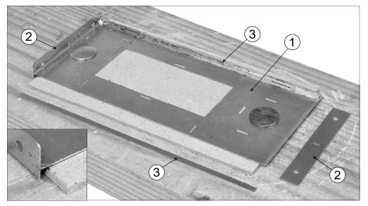
2. Trim the valances (parts 3) to be a slightly loose fit between the buffer beams (this is to prevent the valances buckling when they expand due to the heat of soldering into place). Then solder each valance upright along the footplate edges just outboard of the tank side slots. Once fitted I would recommend cutting a piece of flat softwood so that it fits between the buffer beams and valances to provide a flat solid support for the footplate as construction progresses.
