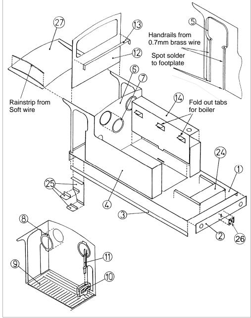
3. Pre form and then solder a length of beading (parts 5) around the cab openings. You will notice that there are three sets of beading and this is because I can never determine the exact length required until I test build the first sample model so I try three slightly different lengths. I find that the medium length fits the best.
