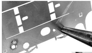
First using your large tapered reamer gently open out the axle holes so that the turned bearings are a good snug fit into them.
