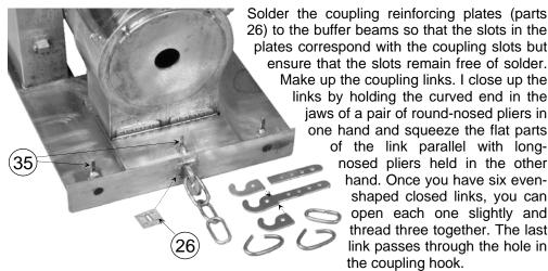
I reinforce the joint of each link with a spot of 60/40 solder. Pass the tail of the hook through the buffer beam slot and then solder solid to the rear of the buffer beam. Then snip off the tail of the coupling.
