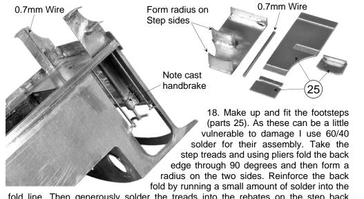
fold line. Then generously solder the treads into the rebates on the step back plates. Fold the top through 90 degrees and reinforce with solder. This top fold fits against the back of the valance and will position the steps the correct distance inboard. To add extra strength I also solder (quickly using 145° solder so that the treads don't fall off) lengths of 0.7mm brass wire to the rear of the back plates.
