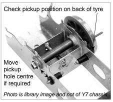
13. Fold chassis and spacers through 90° then fit spacer part 29.
